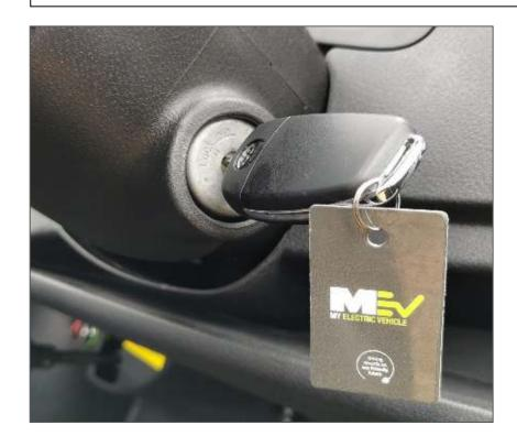
Ignition key needs to be in the off position or removed while charging process takes place
